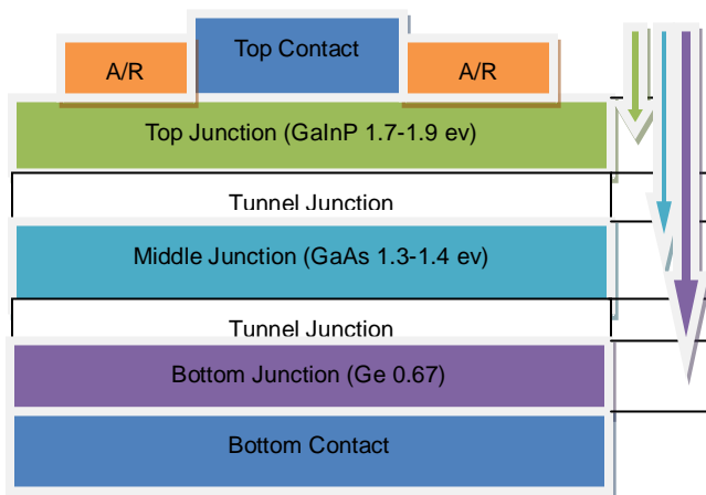
Fig 4: The Internal diagram of a multi-junctioned solar cell.
